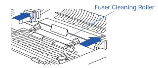
4. Remove the jammed paper by pulling it from the **bottom of the fuser**, through the printer's Back Cover, not from the top of the Fuser area. This prevents any unfused toner from dirtying the Fuser Rollers (located under the Fuser Cleaning Roller).
